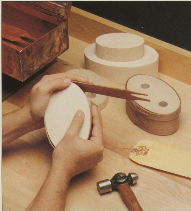
Made from quartersawn cherry veneer, the band for the box shown above is bent around a drying form after first being soaked in hot water and softened. The band is secured in its bent shape by copper tacks.
