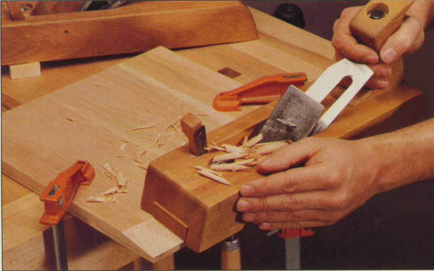
A panel-raising plane bevels one end of a wood panel. These hand tools must be used in pairs to raise a panel. Using left- and right-hand models allows the panel to be beveled in the direction of the grain at all times.
